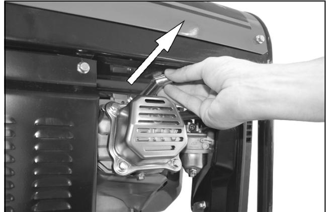
2. Use the spark plug spanner supplied to remove the spark plug.
