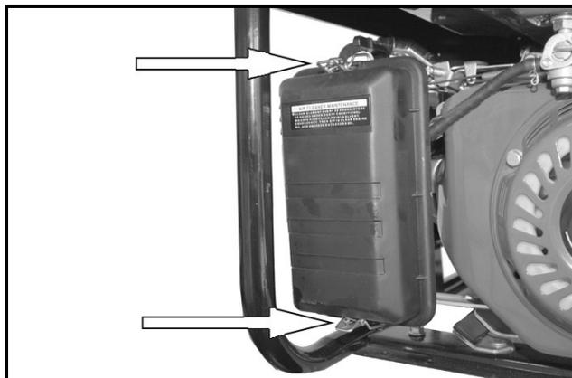
2. Remove the air filter element.
